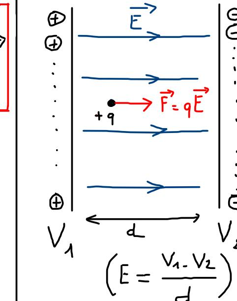
$$\begin{aligned} \epsilon_{p_2} - \epsilon_{p_1} &= - \int_1^2 q \vec{E} \cdot d\vec{P} \\ V_2 - V_1 &= - \int_1^2 \vec{E} \cdot d\vec{P} \end{aligned} \quad \left. \begin{array}{l} \boxed{V = \frac{\epsilon_p}{q}} \\ \text{potentiel électrique} \\ \text{en } V = J \cdot C^{-1} \end{array} \right\}$$
