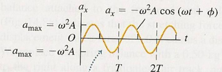
The  $a_x$ - $t$  graph is shifted by  $\frac{1}{4}$  cycle from the  $v_x$ - $t$  graph and by  $\frac{1}{2}$  cycle from the  $x$ - $t$  graph.
