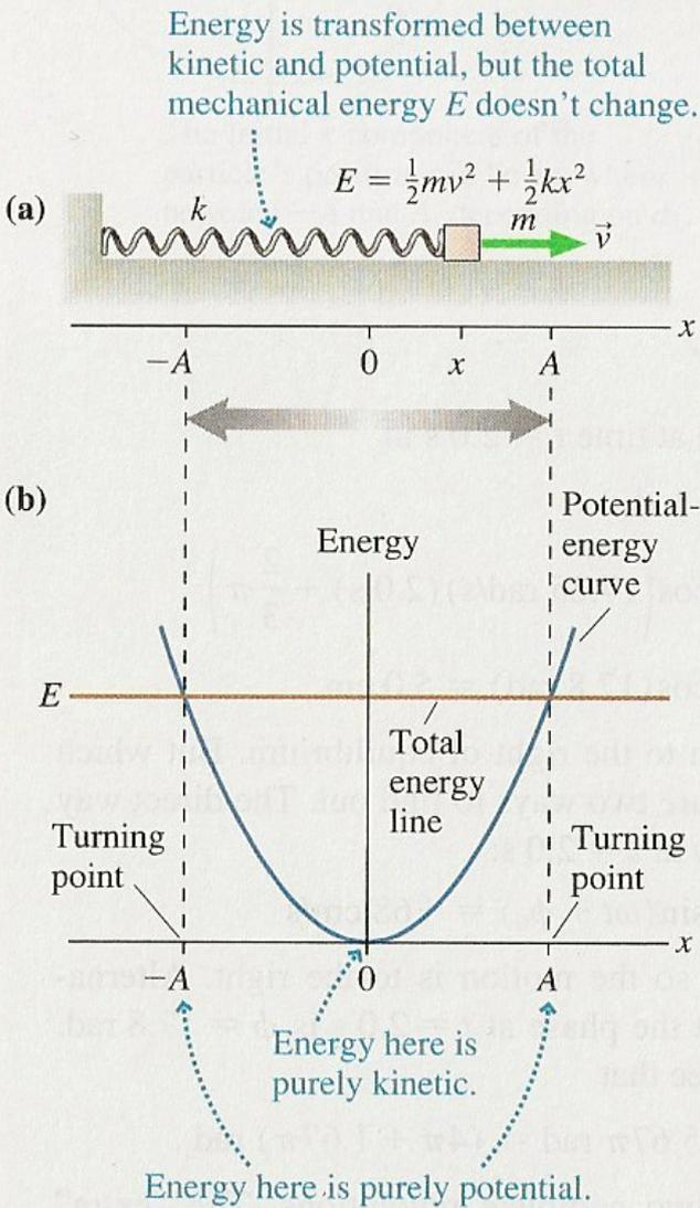
**FIGURE 14.11** Kinetic energy, potential energy, and the total mechanical energy for simple harmonic motion.
