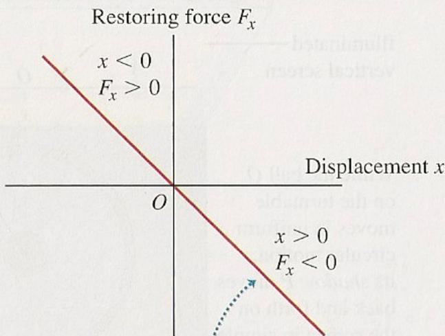
The restoring force exerted by an idealized spring is directly proportional to the displacement (Hooke's law,  $F_x = -kx$ ): the graph of  $F_x$  versus  $x$  is a straight line.
