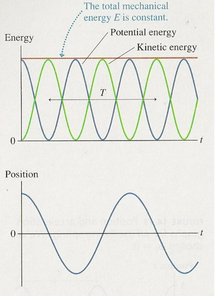
**14.14** Graphs of  $E$ ,  $K$ , and  $U$  versus displacement in SHM. The velocity of the body is *not* constant, so these images of the body at equally spaced positions are *not* equally spaced in time.
