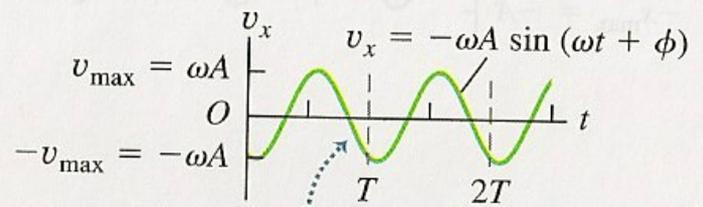
The  $v_x$ - $t$  graph is shifted by  $\frac{1}{4}$  cycle from the  $x$ - $t$  graph.
