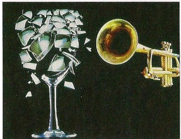
**FIGURE 14-24** This goblet breaks as it vibrates in resonance to a trumpet call.
