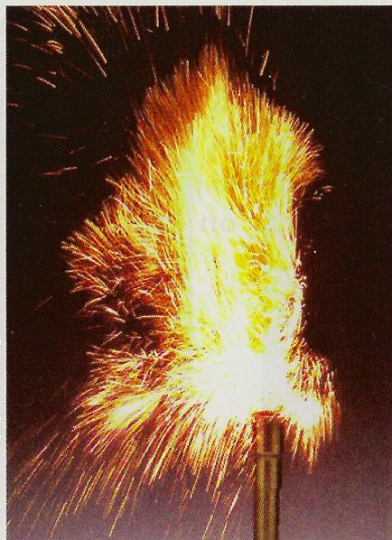
(a) Reaction of iron and oxygen to give iron(III) oxide,  $Fe_2O_3$ .
